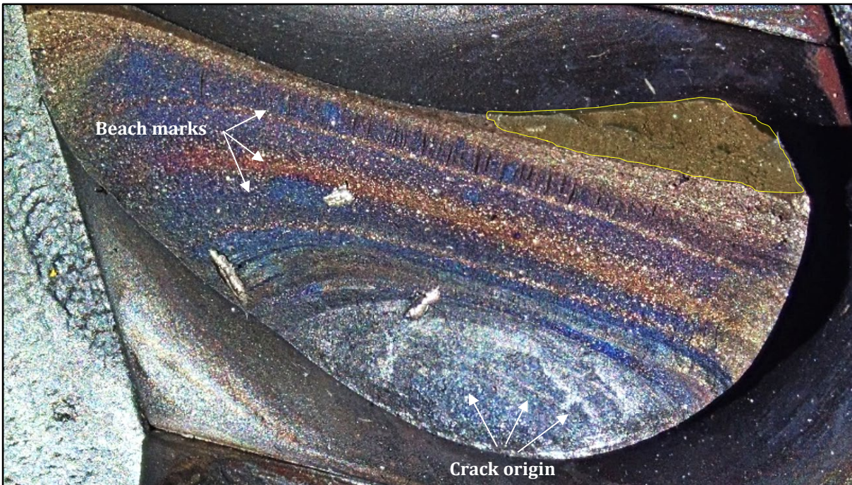
Figure 1. Fracture surface of the blade root, shows a large number of beach marks.
